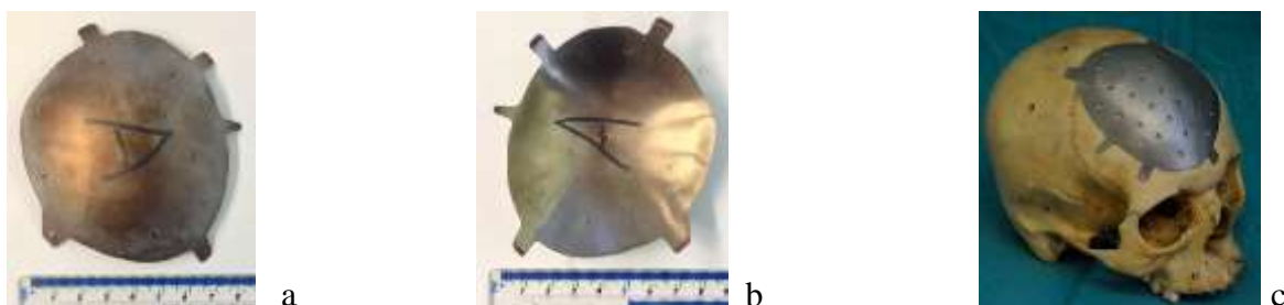
Fig 1. Cranial implant made by ISF: a) front side of the implant; b) back side of the implant; c) human skull.
